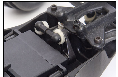
Angled bellcrank co-planar steering with built-in servo saver.
