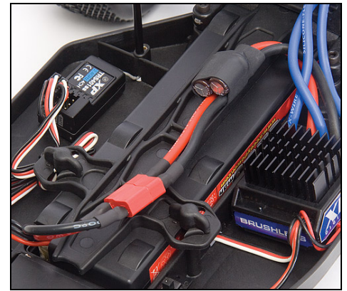
Battery strap with twist-lock thumb knobs.
